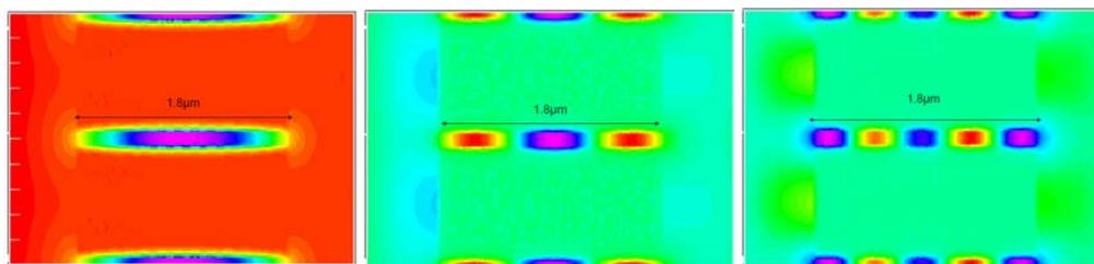
**Figure 2:** Magnetic field  $B_z$  distribution (red: high; blue/pink: low) obtained from simulation for the structure excited with frequencies corresponding to 1<sup>st</sup>, 3<sup>rd</sup> and 5<sup>th</sup> resonant transmission peaks. Standing wave structure inside the slot can be identified.
