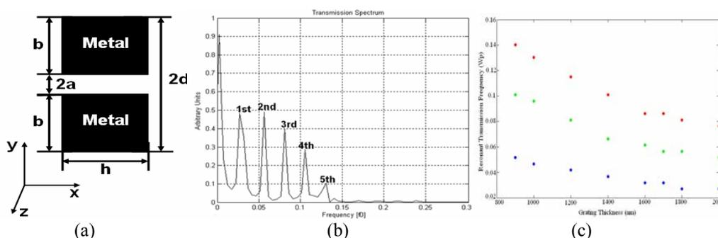
**Figure 1:** (a) Geometry of the modeled plasmonic structure with sub-wavelength periodic grating. (b) Spectrum of extraordinary transmission through the aperture array, the frequency has been normalized to plasma frequency. Five frequency peaks correspond to five resonant transmission modes. (c) First three resonant frequencies scale nearly linearly with grating thickness.
