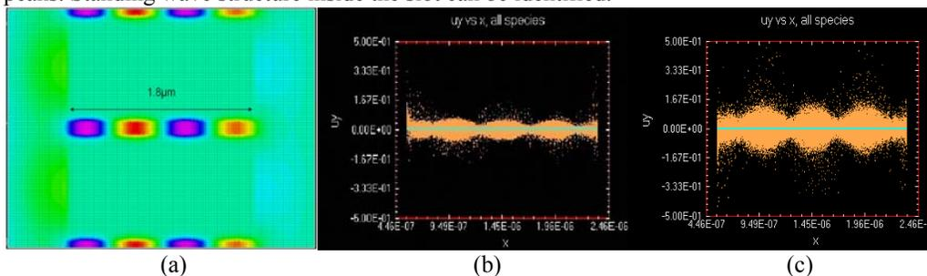
**Figure 3:** (a) Magnetic field  $B_z$  distribution for the structure excited by the frequency corresponding to the 4<sup>th</sup> resonant transmission peak. (b, c) Snap-shot of distributions of particle velocity  $V_y$  inside the metal the along the slot. Panels b,c correspond to different instants.  $V_y$  is oriented along the direction of electric field of TM mode EM wave.
